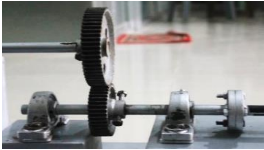
Fig. 1. Geared power transmission for offset shafts [5].
